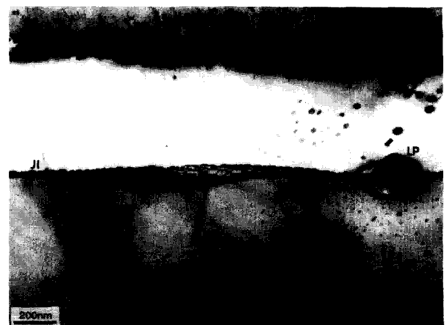
Fig. 4. Cross-sectional TEM image in bright field at the joining interface. The upper and lower sides of the joining interface indicate the Cu-implanted and non-implanted samples. The symbols: JI, LP, and SP are the joining interface, large precipitate on the dislocation networks, and small precipitates, respectively.
