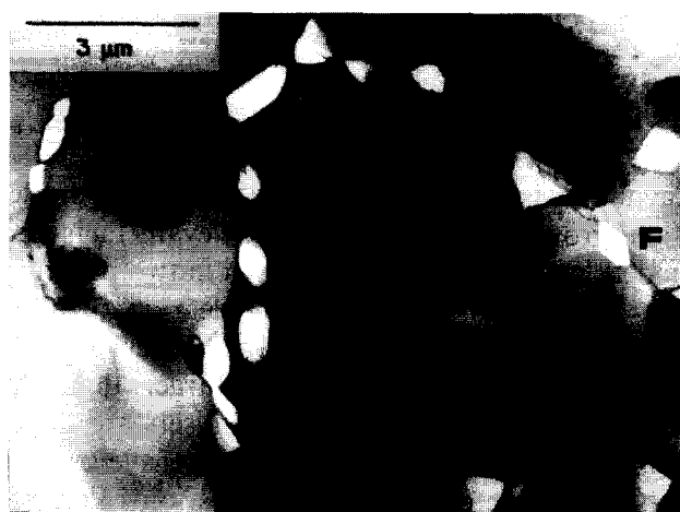
Fig. 4. Faceted cavities (F) in AlN after creep in compression ( T = 1873 \text{ K} , \sigma = 250 \text{ MPa} , \epsilon = 2.3 \times 10^{-2} ). Dislocations (D) and one inversion domain boundary (I) can be seen in one grain.
