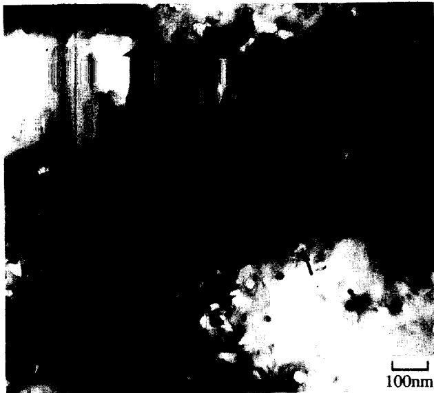
Fig. 7. TEM bright-field micrograph of a powder A compact sintered at 1250°C for 2 h showing the presence of micro-pores (some arrowed) scattered in the material.
