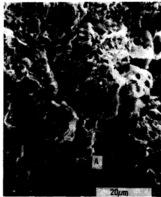
Fig. 7. Fracture surface of material aged for 32 h fractured at room temperature. Note that although there is some crack-precipitate interaction present, the fracture is predominantly inter-granular, and that there are regions of grain boundary monoclinic phase (A) through which the crack has preferentially propagated.
