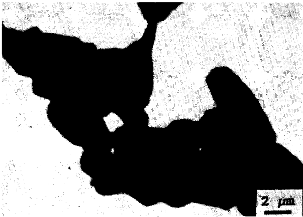
Fig. 3. Backscattered SEM ECP micrograph of ER RS Si-SiC composites: silicon and polycrystalline silicon carbide (35 vol%). SiC grain exhibits different orientations.
