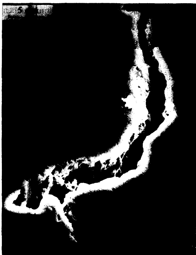
Fig. 3. A typical cracklike defect is presented on the surface of pressureless sintered ZY5 samples.
