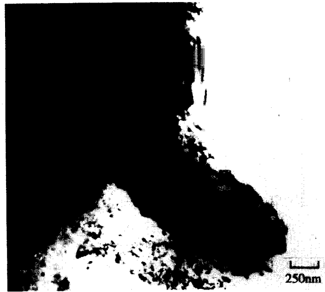
Fig. 8. TEM bright-field micrograph of a powder A compact sintered at 1275°C for 2 h showing that pores present in the diphasic matrix are engulfed by mullite grains. White features inside the black mullite grain (M) are the pores.
