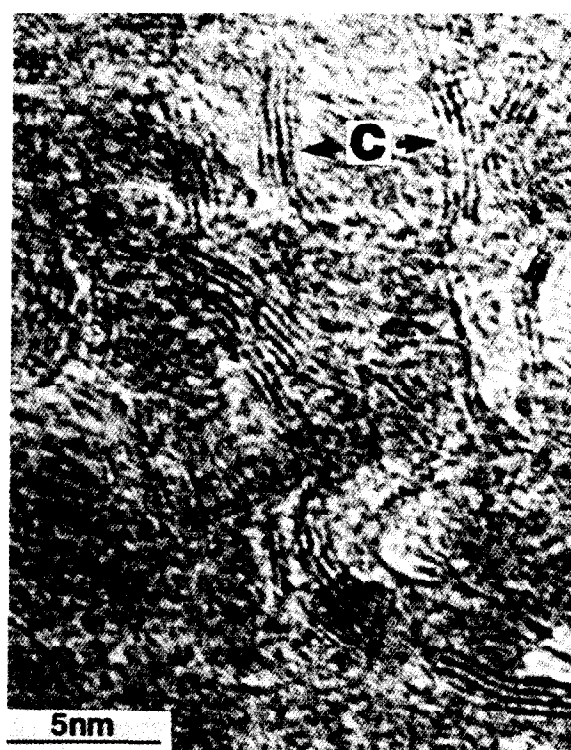
Fig. 3. LF image of distorted graphene stacks obtained from the removal of peripheral hydrogen atoms of BSUs and subsequent BSU edge-to-edge association (example taken from a PCSZ-based Si-C-N ceramic with x = 0.1 ).
